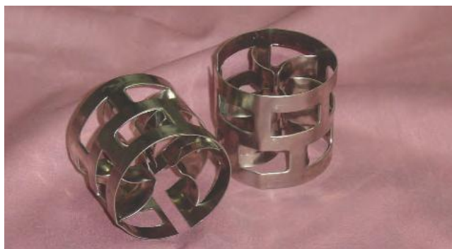
The low-aspect-ratio of CASCADE MINI-RINGS ® high performance random packing (Top) favors orientation which exposes internal surfaces for excellent liquid film formation, intimate mixing and vapor/liquid contact. The high-aspect-ratio of the Pall-Ring random packing (Bottom), on the other hand, permits occlusion of interior surfaces and increased pressure drop.
